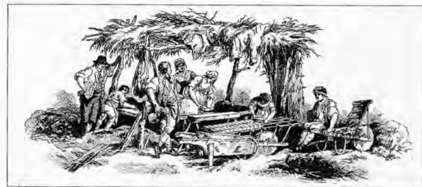
Fig.6 Brickmaking c.1800: Men, women and children brickmakers, perhaps all members of the same family, at work in a crudely thatched temporary hovel. To the left, a young boy is placing a lump of pugged clay on the moulding table, while, beside him, the man in the hat is probably the brick moulder. In the centre a young woman is taking a moulded brick on a stock board, ready to be loaded by the young girl, to the right, onto a barrow. When fully loaded, this will be wheeled off to the drying hacks. (W.H. Pyne, Microcosm , 1808, p.210, Plate 125, Fig.2)
